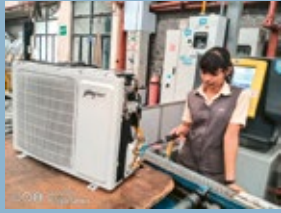
6. Leak Detection after Charging
