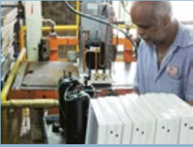
1. Srew Removal, Earth Wiring, Compressor Fitting
